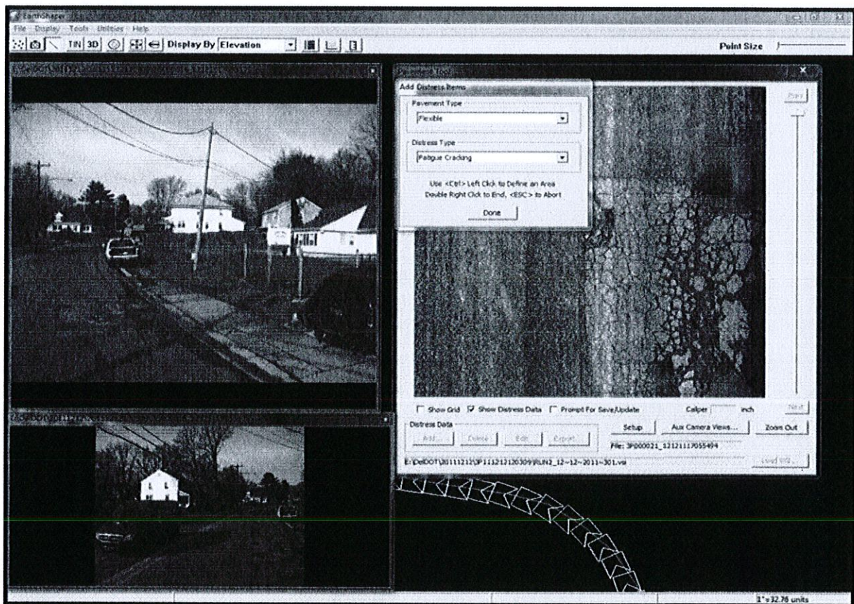
Pavement Condition Evaluation within EarthShaper™ software
