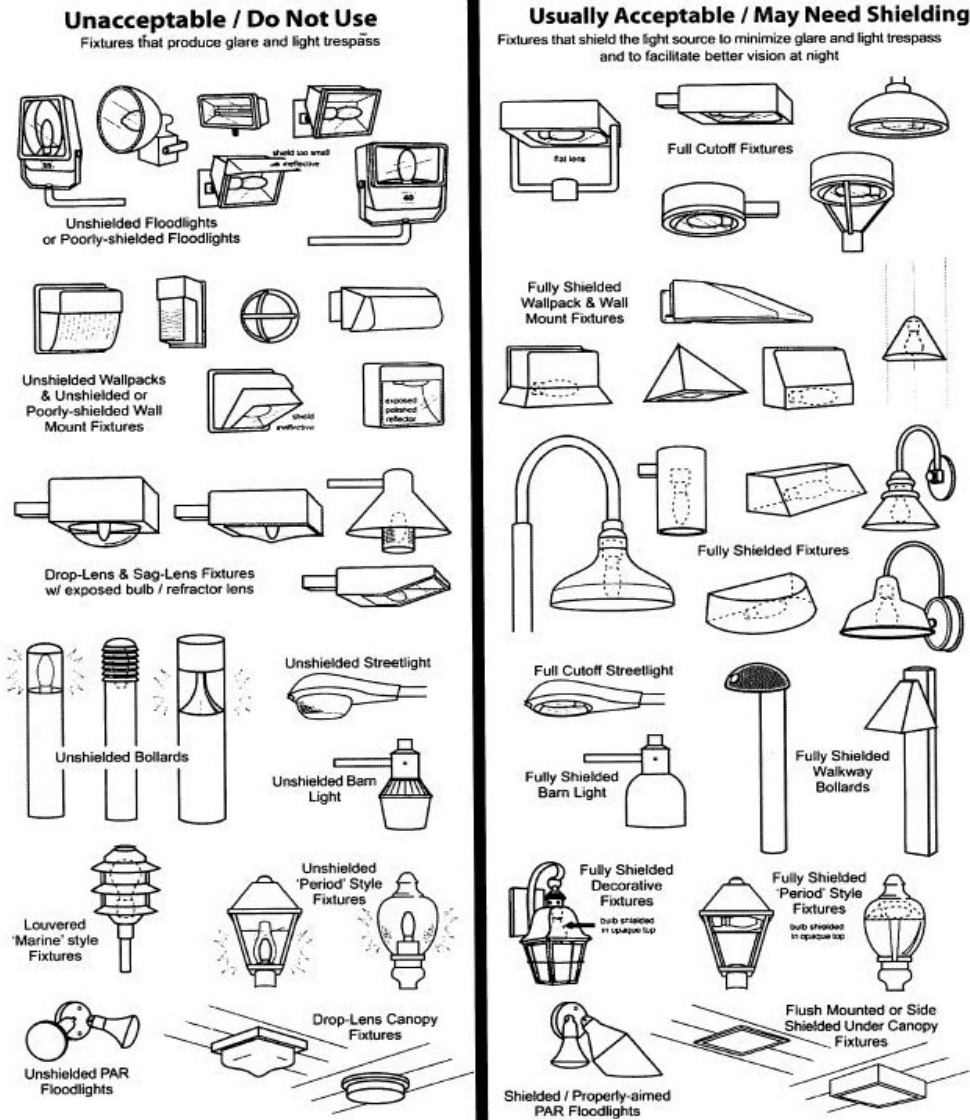
Figure 3.8-4 Unacceptable Fixtures and Fixtures Requiring Shielding
