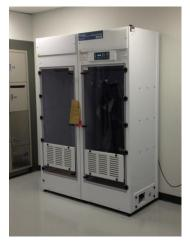
your evidence from airborne pathogens and cross-contamination while eliminating personnel exposure to putrid odors of decomposition and harmful bacteria or viruses. The unit is configured to clean the incoming "drying" air through pre-filtration and then filter the cabinet exhaust air through a combination of bonded carbon and HEPA filtration.
